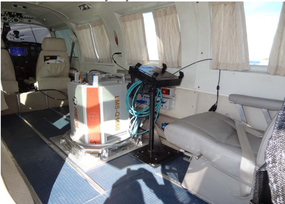
View above and below of modified interior and 21" X 21" Camera hole
