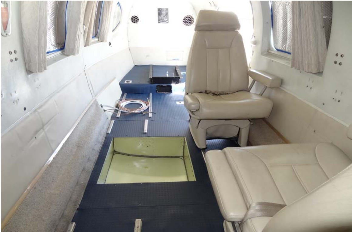
View above and below of modified interior and 21" X 21" Camera hole
