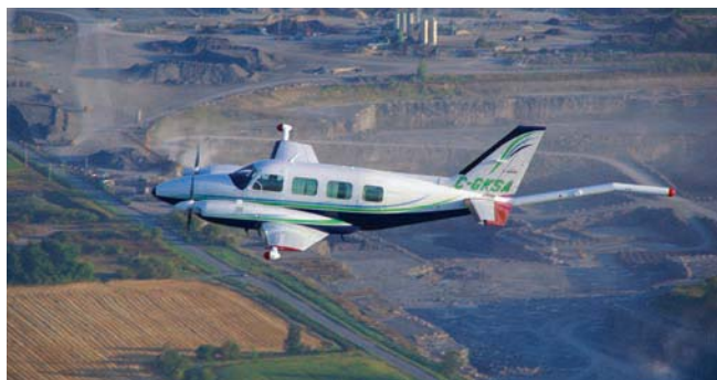
KASI Aviation's horizontal magnetic gradiometer system showing wing-tip pods and tail stinger Credit: KASI Aviation Services
